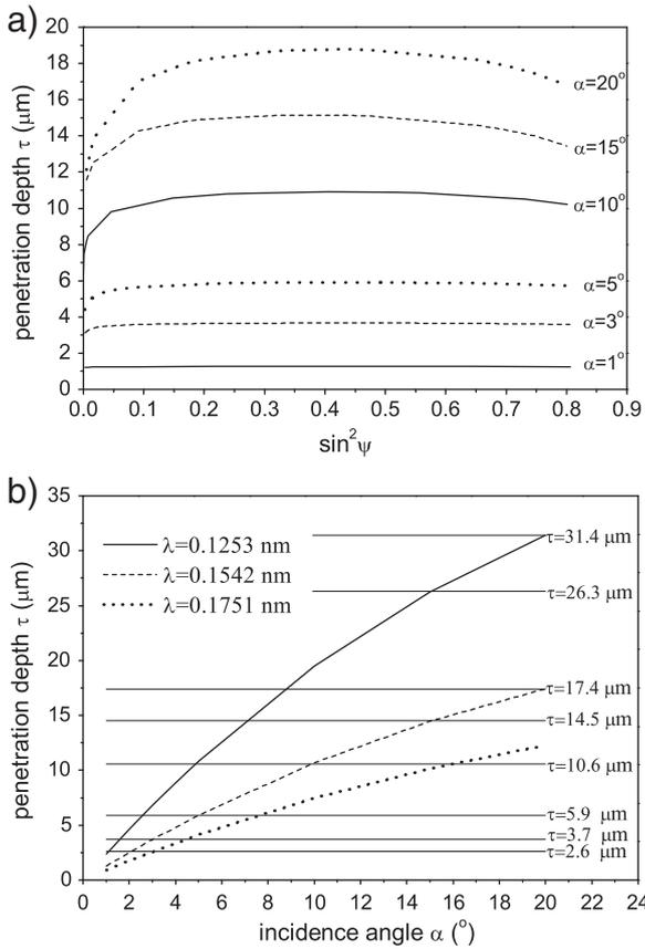
**Fig. 2.** The penetration depth ( $\tau$ ) vs.  $\sin^2 \psi$  of X-rays in Al sample for different incidence angles and constant wavelength  $\lambda = 1.54056$  (a), and the dependence of  $\tau$  vs.  $\alpha$  for three different wavelengths used in the experiment (b). Calculations were performed for MGIXD geometry according to Eq. (2) ( $\alpha \gg \alpha_{cr} = 0.23^\circ$ ).
