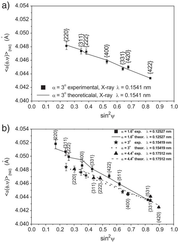
Fig. 3. Measured lattice parameters  $\langle a(\phi, \psi) \rangle_{\{hkl\}}$  (points) and theoretical results of fitting (continuous lines) vs.  $\sin^2\psi$  for polished Al samples. Results of grazing incidence method obtained from classical diffractometer (a) and from synchrotron radiation (b) are presented. The plots are shown for the penetration depth  $\tau = 3.48$   $\mu\text{m}$ .
