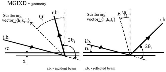
**Fig. 1.** Geometry of MGIXD method. The incidence angle  $\alpha$  is fixed during measurement, while the orientation of the scattering vector is characterized by the angle  $\psi$  (where  $\psi(hkl) = \theta(hkl) - \alpha$ ).
