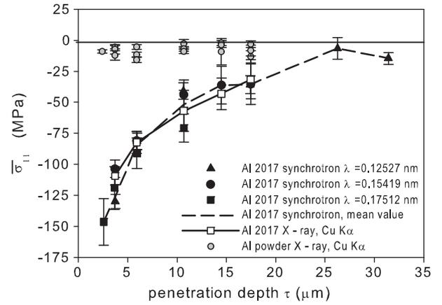
Fig. 4. Experimental  $\bar{\sigma}_{11}$  stress in function of penetration depth  $\tau$  for polished Al2017 sample and Al powder. Results obtained from laboratory diffractometer (Cu  $K\alpha$ -radiation) and using synchrotron radiation with three different wavelengths are compared.
