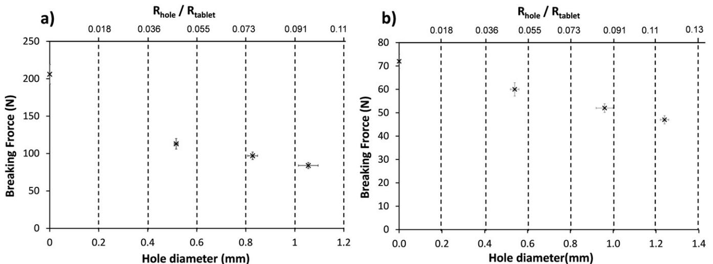
**Fig. 4.** Breaking force in the diametral compression test, as a function of the hole size: (a) SDLac and (b) aCP. The upper axis represents the ratio between the hole radius ( $R_{\text{hole}}$ ) and the tablet radius ( $R_{\text{tablet}}$ ).
