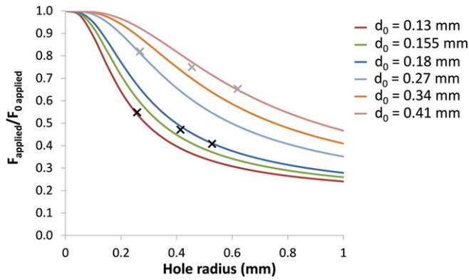
**Fig. 6.** Application of the point stress criterion. The graph represents the ratio between the force needed to break a compact with a hole and the force needed to break a compact without a hole as a function of the hole radius. Continuous lines are obtained according to Eq. (12) for several values of  $d_0$ . Marks represent the experimental values: (x) SDLac and (x) aCP.
