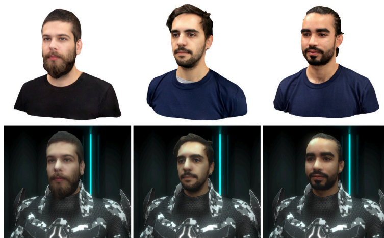
FIGURE 1 | Illustration of three raw bust models (50K polygons) and of their optimized versions (2.5K polygons) integrated in the virtual reality application. Written informed consent was obtained from the depicted individuals for the publication of this image.
