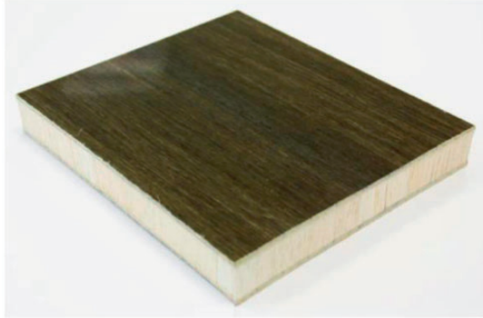
Figure 1. Flax/Elium/Balsa sandwich panel.
