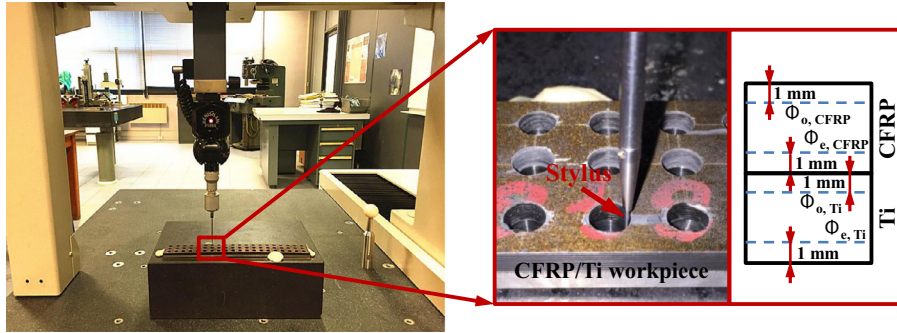
Fig. 3. Photograph showing the process setup of hole dimensional feature measurement.
