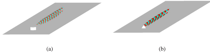
Fig. 3 Streamwise velocity component of the eigenvector of the most unstable mode obtained at Re = 1000 for the cylindrical roughness element (a) and the smooth one (b).
