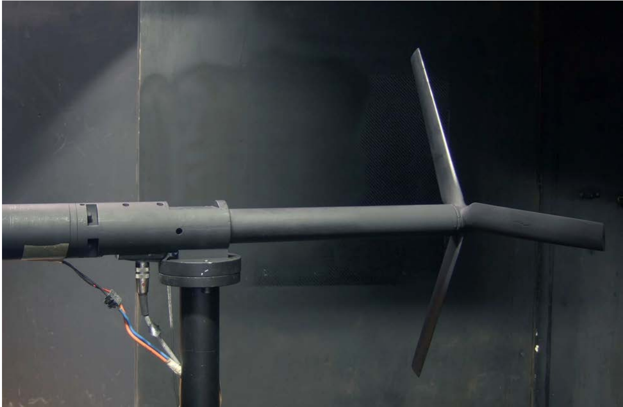
FIG. 15: Tested wind turbine in the wind tunnel
