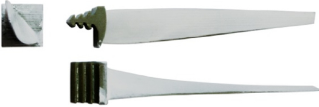
Fig. 4. 3D printed blades view: top, pressure side, leading edge side.
