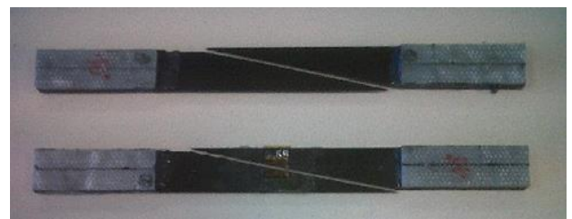
Figure 8 10^\circ Shear failure
