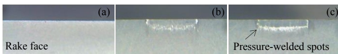
Fig. 6. Direct observation of the tool's rake surface after cutting Sn under different gas shields: (a) Argon; (b) Room ambient; (c) Oxygen
