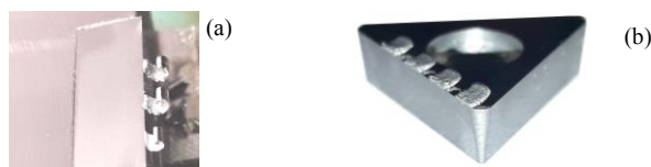
Fig. 7. Direct observation of the chip curling of Tin (Sn): (a) Inert gas shield of Argon; (b) Active gas shield of Oxygen. Test parameters: polished tool, t_0=0.025\text{mm} , w=2\text{mm} , V_c=500\text{mm/min} .
