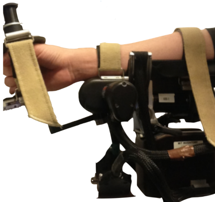
Figure 1. Massachusetts Institute of Technology Wrist-Robot and experimental forearm, wrist, and hand position (excluding finger strap).
