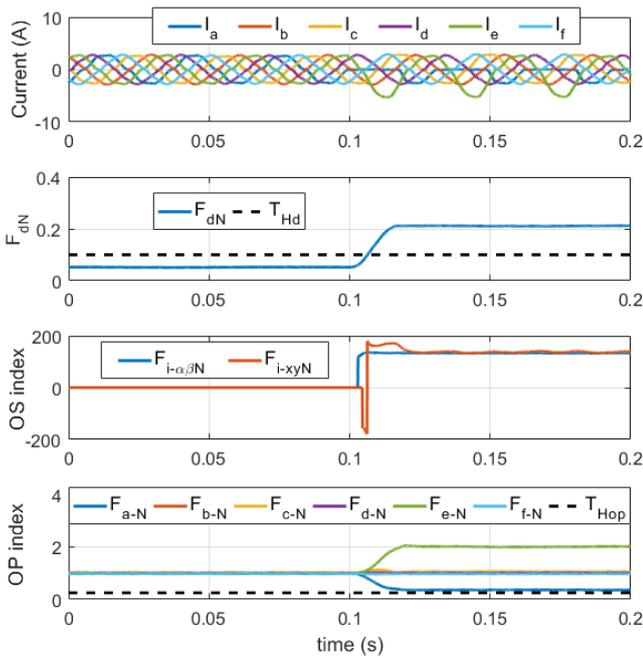
**Fig. 14.** Experimental results of the diagnostic algorithm effectiveness. Time-domain waveforms of the phase currents and the diagnostic variables when an open-circuit fault occurs in transistor T1.
