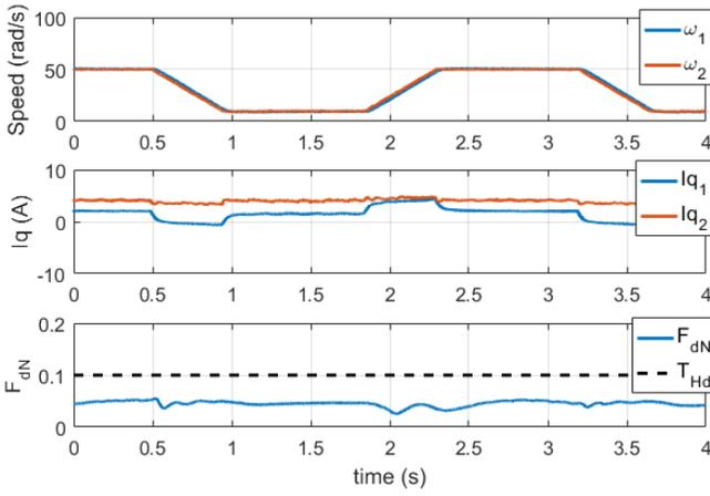
**Fig. 11.** Experimental results of the diagnostic algorithm immunity to false alarms. Time-domain waveforms of the phase currents, the rotor speeds of the two series-connected machines and the diagnostic variables during speed change.
