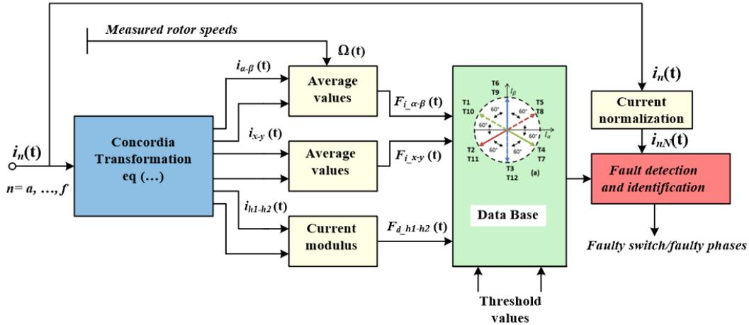
Fig. 8. Block diagram of the proposed diagnostic algorithm.
