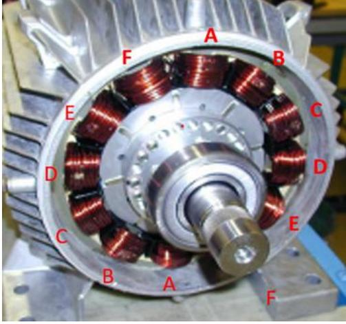
Fig. 2. Symmetrical six-phase 12-winding PMSM.
