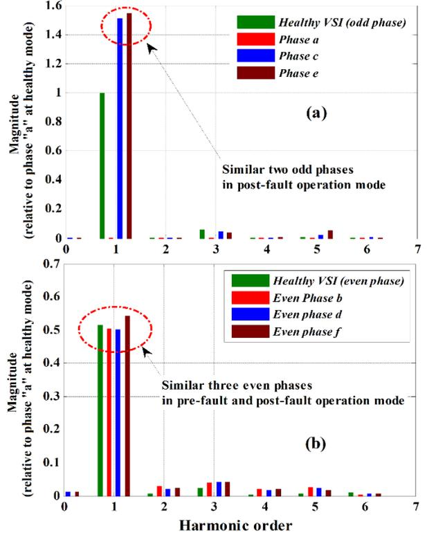
**Fig. 7.** Experimental results: harmonic contents of the phase currents for a normal operation mode and under an open-phase fault (motor phase a opened). (a) Odd phase currents a, c, e. (b) Even phase currents b, d, f.
