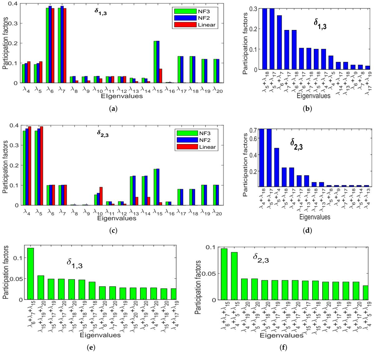
**Figure 5.** (a) 1-eigenvalue mode-in-state participation factors to machine 1 relative angle. (b) 2-eigenvalue participation factors to machine 1 relative angle. (c) 1-eigenvalue participation factors to machine 2 relative angle. (d) 2-eigenvalue participation factors to machine 2 relative angle. (e) 3-eigenvalue participation factors to machine 2 relative angle. (f) 3-eigenvalue participation factors to machine 2 relative angle.
