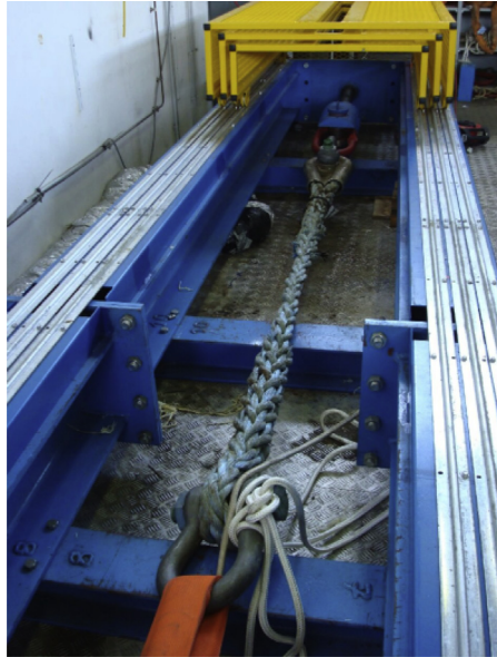
Figure 14.8 Residual tensile strength test on rope sample on a 1000 kN capacity test frame.
