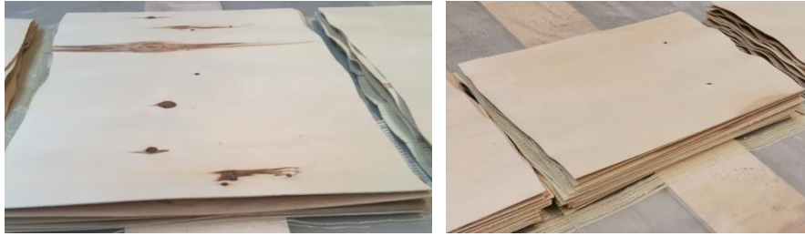
Figure 3. Veneers used in the paneling process. Left: Low quality veneers for Q2 panels. Right: High quality veneers for Q1 panels.
