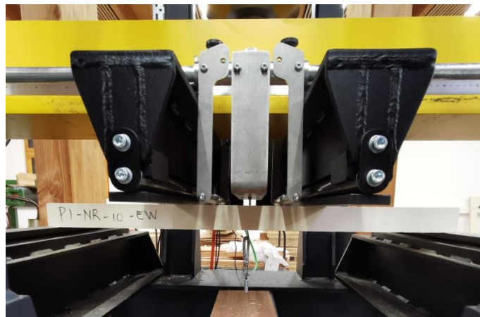
Figure 8. LVL poplar beam during bending test.
