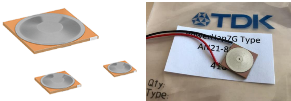
Figure 3: TDK PowerHap piezoelectric actuators.
