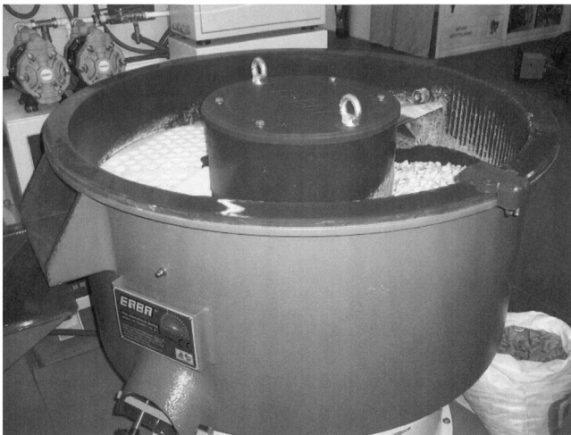
Figure 5. Vibro-abrasive machine (Erba Company) with ceramic shaped stones used for finishing of aircraft alloys (Marbad Ltd. Company, Warsaw, Poland).
