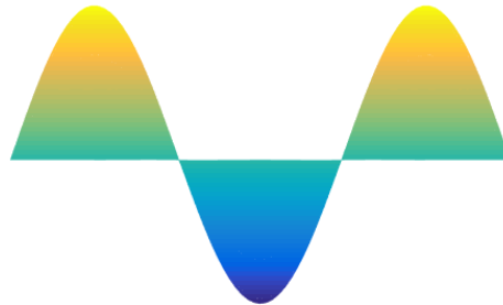
Figure 9: Deformed shape at point E of Figure 8. The plate has switched to mode 3, as in the point D of Figure 7.
