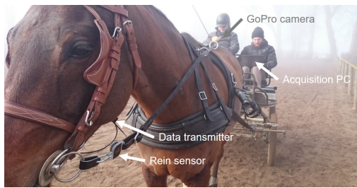
Fig. 11. Setup for the data collection with the rein sensor attached to the reins.
