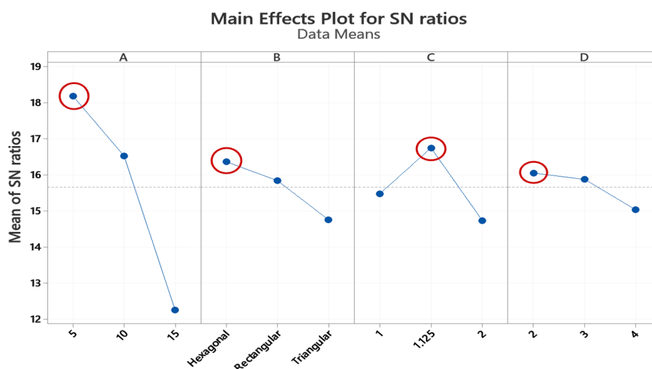
Figure 4. Main effect plot cylindricity. A, B, C, and D represent the Thickness, Infill Pattern, Layer height, and Wall Layer, respectively.
