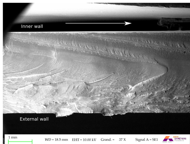
Figure 9. Observation by electron microscopy of the propagation zone of the fracture surface of sample PS2-33. The arrow indicates the direction of propagation.
