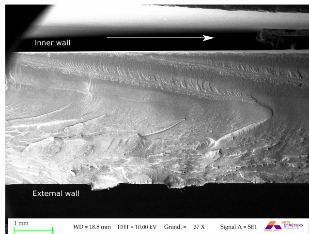
Figure 9. Observation by electron microscopy of the propagation zone of the fracture surface of sample PS2-33. The arrow indicates the direction of propagation.
