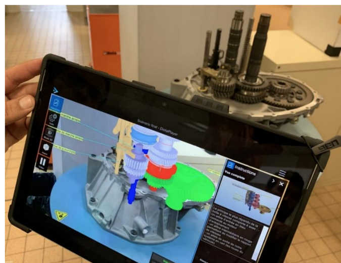
Figure 15. AR Hololens car gearbox scenario.
