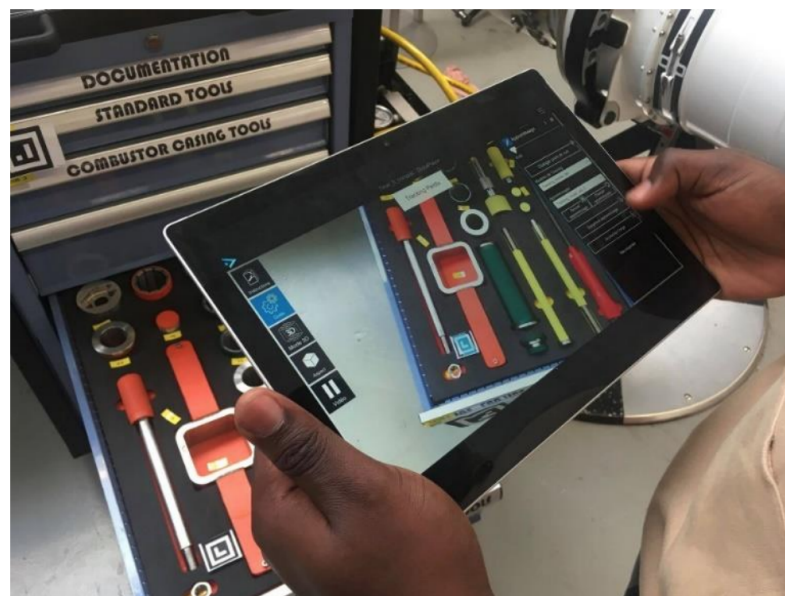
Figure 9. Identification of a tool in the tool trolley, during the AR scenario.
