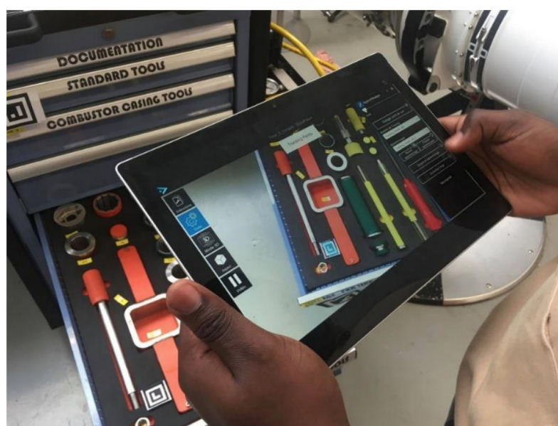
Figure 9. Identification of a tool in the tool trolley, during the AR scenario.
