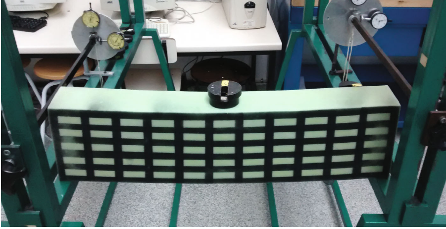
FIGURE 1 A view of the foam beam at the lab. It consists of a simply supported beam whose constitutive behavior is known to fit well to a Kirchhoff–Saint Venant law. The thick black lines help to track selected points in the image
