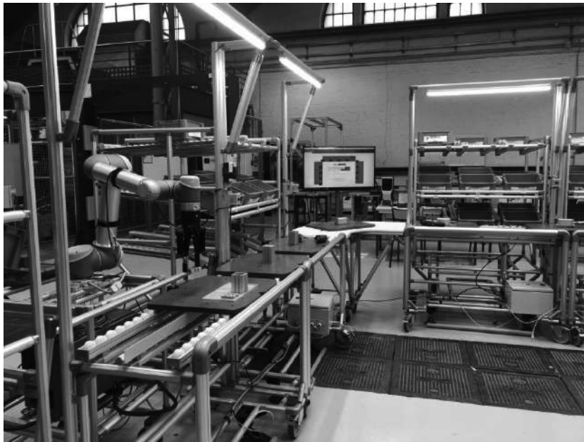
Figure 11.5. Line equipped with 4.0 technologies (collaborative robot, RFID, interactive dashboard)
