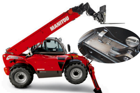
Fig. 1. Telehandler Manitou MT1840 and a closer view of typical welded connections found on the chassis.
