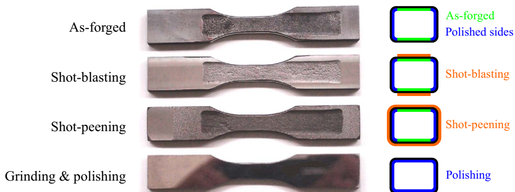
Fig. 3. Specimens from each batch with cross-section detailing the specimen preparation.
