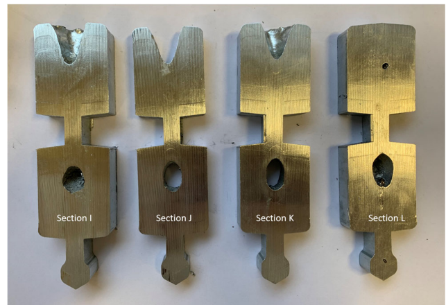
Fig. 12 Pictures of some planes showing macro-shrinkage formation
