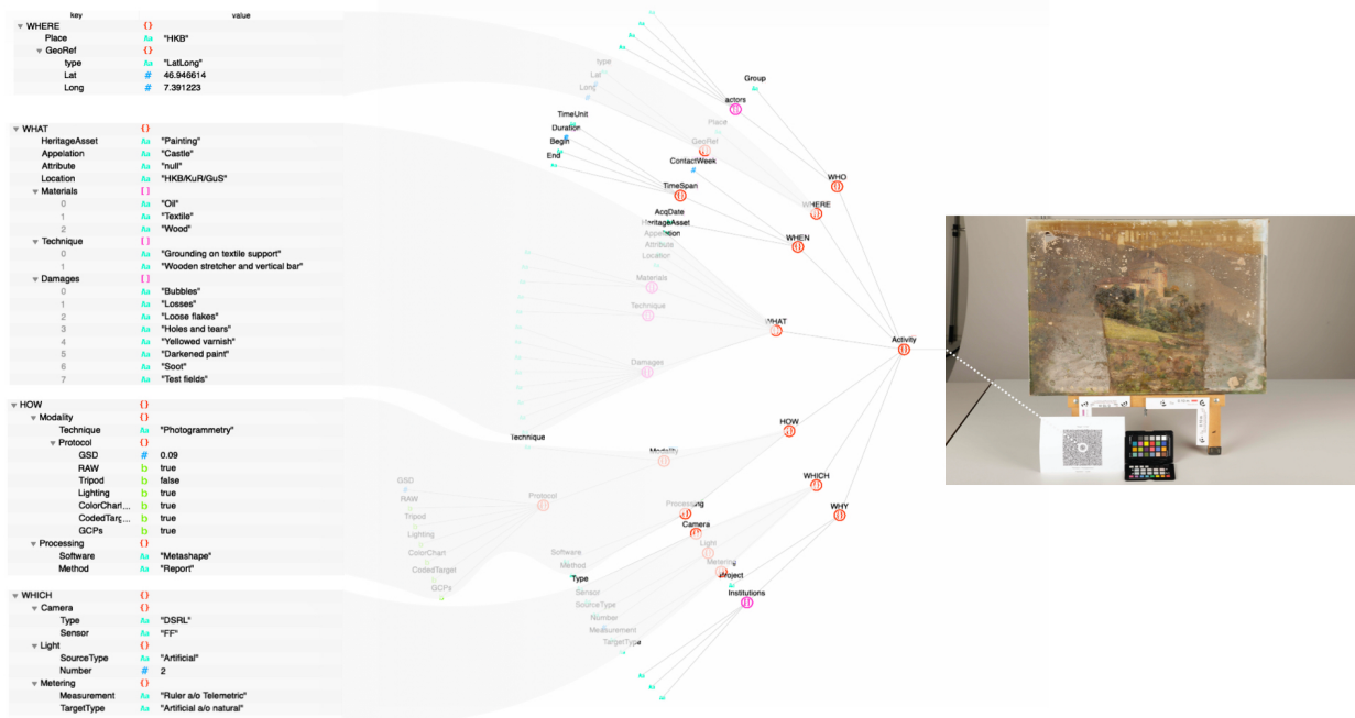
Figure 8. Example of MEMoS QR code and embed metadata captured alongside colorimetric chart prior to photogrammetric acquisition.
