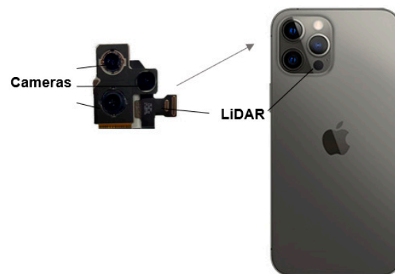
Figure 1. LiDAR system on an iPhone 12 Pro Max.
