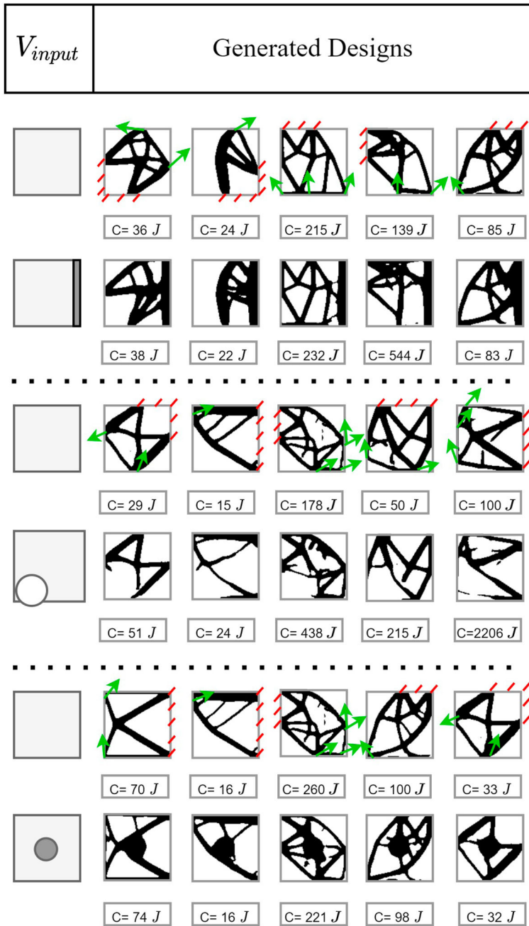
Figure 11. Sample of DL-TO designs generated without versus with constraints on the design area's boundary as input ( V_{input} ). All designs are threshold: (a) additional material is added on the right edge; (b) a hole (passive element) of radius r = 30 is enforced at the bottom left of the design space; (c) an active element of radius r = 15 is enforced at the centre of the design space. The BC (dashes in red) and F (arrows in green) conditions are only shown on the first row. The computed compliance C in Joules ( J ) is shown under the design.
