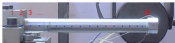
Fig. 9. Scanning points of Vibrometer on the boring bar
