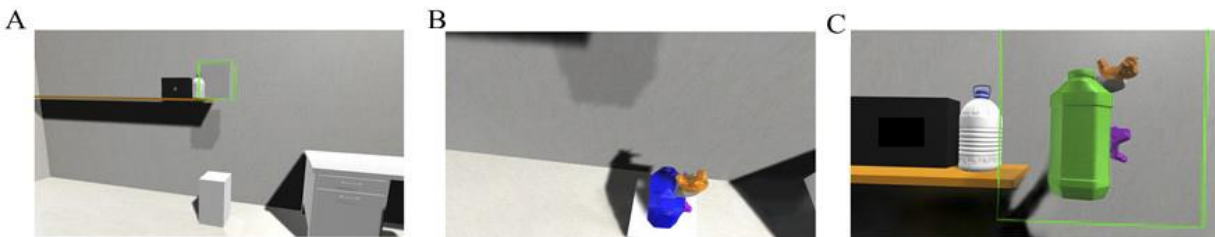
Figure 4. A) Virtual environment displayed in the VR HMD. B) User’s view before starting to lift the bottle, grabbing the bottle (visual feedback in blue). C) View of the end of the task (bottle in green).
