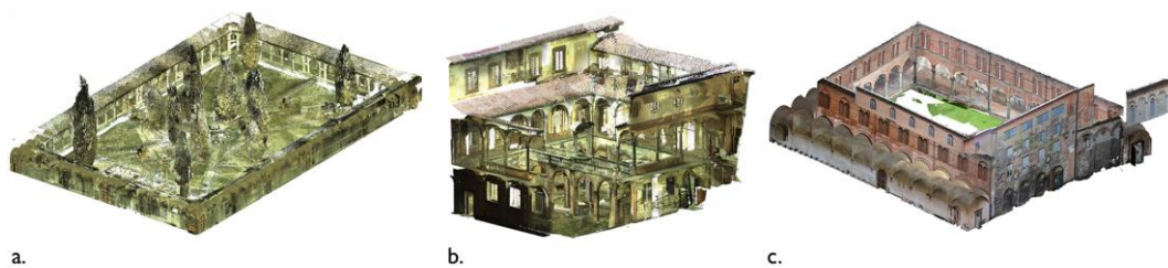
Figure 5. Point clouds for the three case studies considered: the Grand cloister of the Pisa Charterhouse (a); the Grand-Ducal cloister of the Pisa Charterhouse (b); the cloister of the National Museum of San Matteo in Pisa (c).
