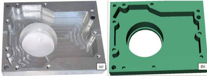
**Figure 8:** The pocket workpiece and its CAD.
