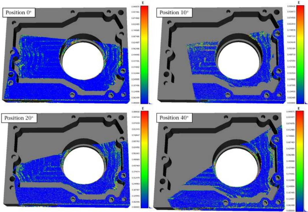
Figure 12: Normal error of the four scans.
