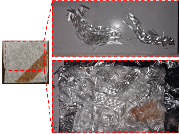
Figure 7: Examples of bent chips retrieved from specimens after matrix burn-off processed from 160x20 mm chips.
