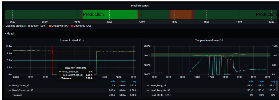
Figure 10. Electrical failure of the band heater (Grafana).
