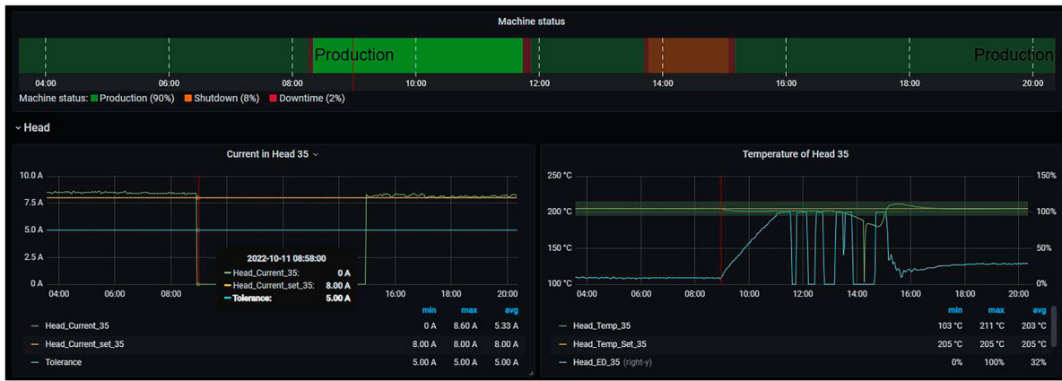
Figure 10. Electrical failure of the band heater (Grafana).
