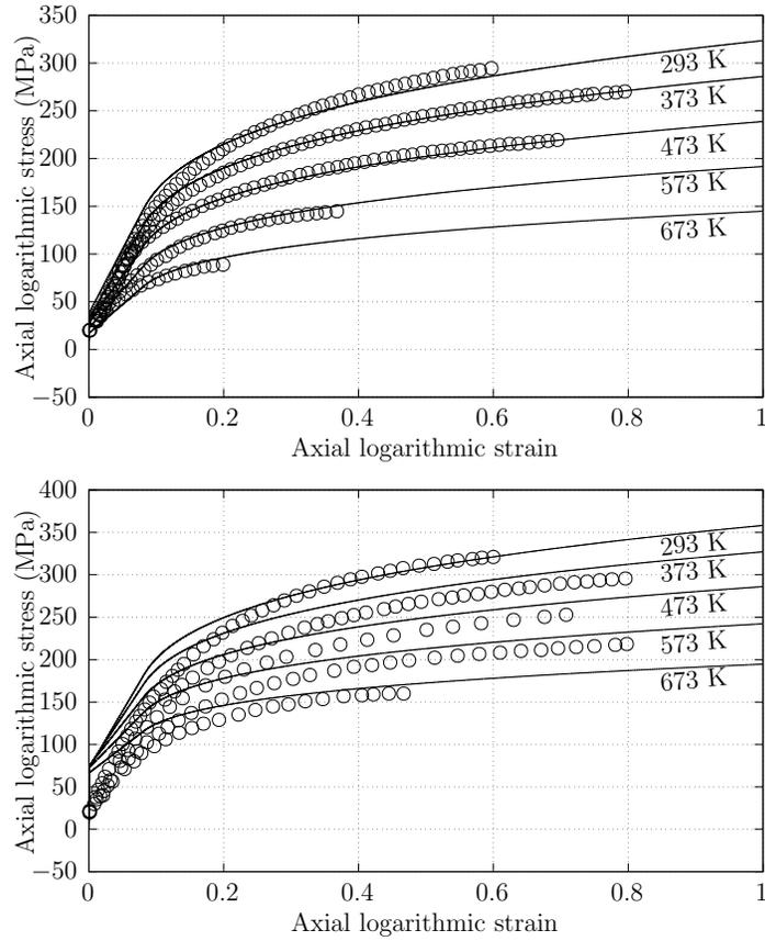
Figure 5: Logarithmic stress-strain curves obtained for polycrystalline copper under uni-axial tension at different temperatures with a strain rate of either  $10^{-4} \text{ s}^{-1}$  (top) or  $1 \text{ s}^{-1}$  (bottom). Dots correspond to the experimental data of Chen and Kocks (1991). Numerical data obtained from the present model is represented with solid lines.
