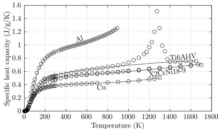
Figure 1: Temperature dependence of the specific heat capacity of several metallic materials. Dots correspond to the experimental data taken from (Miločević and Aleksić, 2012; Ziegler *et al.*, 1963; Kim, 1975; Touloukian and Ho, 1977; White and Collocott, 1984; Brooks and Bingham, 1968). Numerical data obtained from Equation (65) is represented with solid lines.
