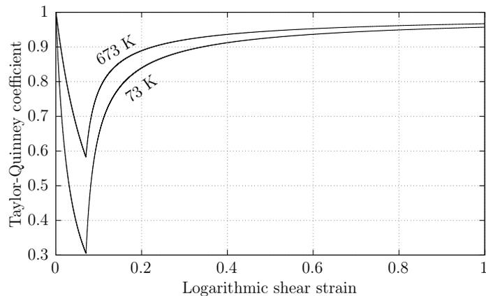
Figure 8: Evolution of the differential Taylor-Quinney coefficient for polycrystalline copper under simple shear with a shear strain rate of  $1 \text{ s}^{-1}$  and a temperature of either 73 K or 673 K.
