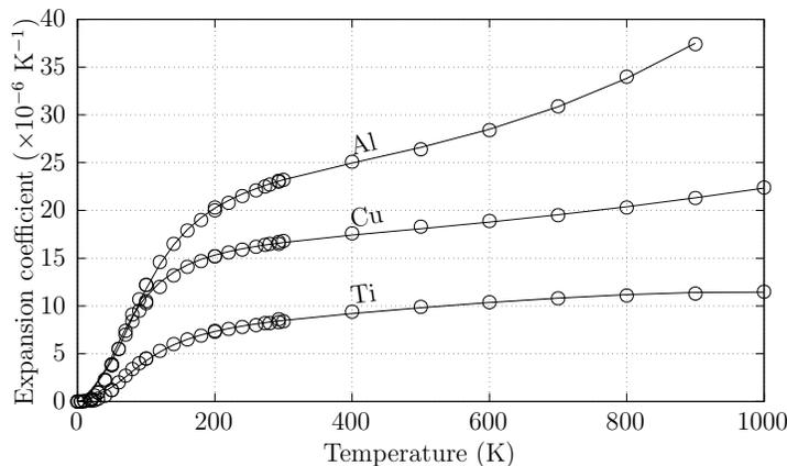
Figure 2: Temperature dependence of the linear thermal expansion coefficient of several metallic materials. Dots correspond to the experimental data taken from (Johnson, 1960; Touloukian *et al.*, 1975). Numerical data obtained from Equation (66) is represented with solid lines.
