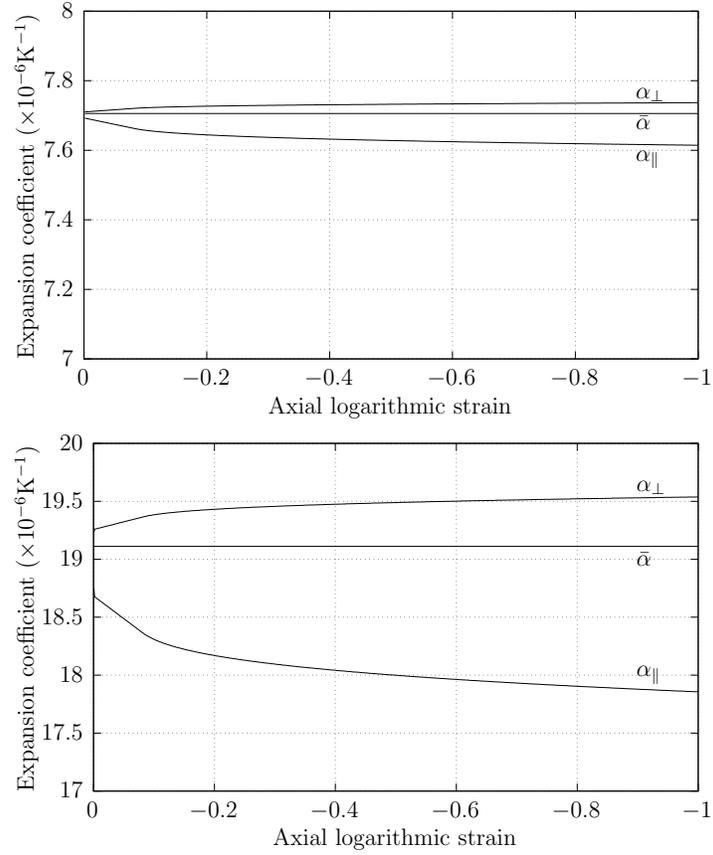
Figure 10: Evolution of the linear thermal expansion for polycrystalline copper under uniaxial compression with an axial strain rate of  $-1 \text{ s}^{-1}$  and a temperature of either 73 K (top) or 673 K (bottom). The linear thermal expansion coefficient parallel and perpendicular to the loading direction are respectively denoted by  $\alpha_{\parallel}$  and  $\alpha_{\perp}$ . The stress-free linear thermal expansion coefficient is denoted by  $\bar{\alpha}$ .
