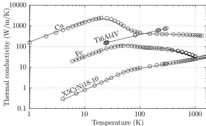
Figure 3: Temperature dependence of the thermal conductivity of several metallic materials. Dots correspond to the experimental data taken from (Touloukian and Ho, 1977; Godfrey *et al.*, 1964; Hust, 1969, 1984). Numerical data obtained from Equations (67) (copper and iron), (70) (X5CrNi18-10 stainless steel) and (71) (Ti6Al4V alloy) are represented with solid lines.
