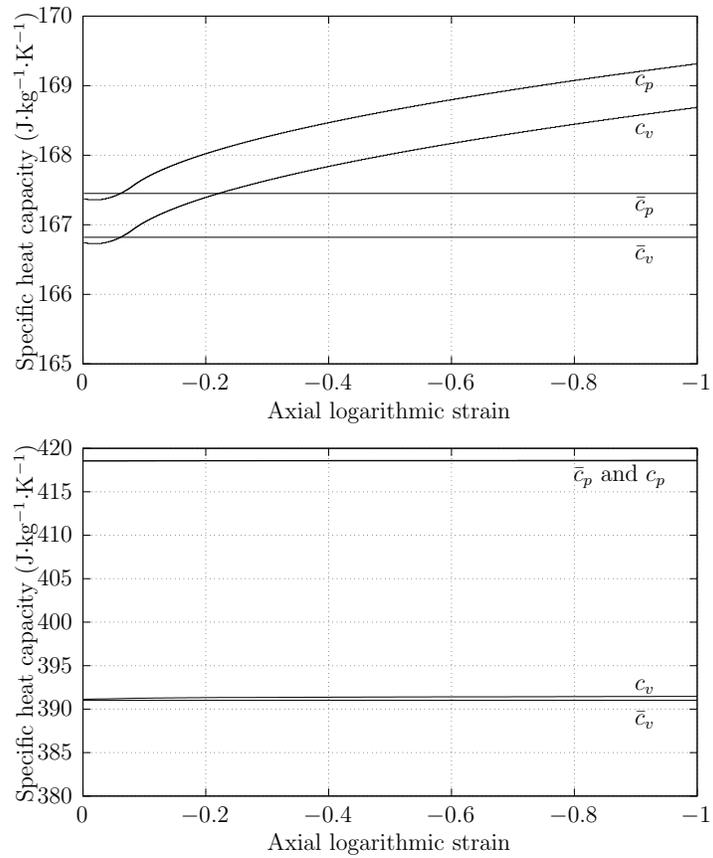
Figure 9: Evolution of the specific heat capacity for polycrystalline copper under uniaxial compression with an axial strain rate of  $-1 \text{ s}^{-1}$  and a temperature of either 73 K (top) or 673 K (bottom).
