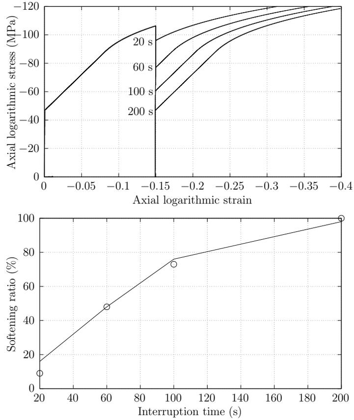
Figure 6: Logarithmic stress-strain curves obtained for polycrystalline copper under uniaxial compression at 723 K with a strain rate of  $0.18 \text{ s}^{-1}$  and different interruption times (top). Evolution of the softening ratio as a function of the interruption time (bottom). Dots correspond to the experimental data of McQueen and Vazquez (1986). Numerical data obtained from the present model is represented with solid lines.
