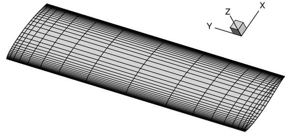
**Figure 3.** Selected mesh for the wing with an aspect ratio of 4.
