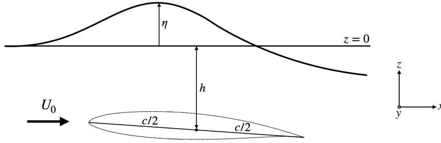
Figure 1. Schematic description of the fluid problem.
