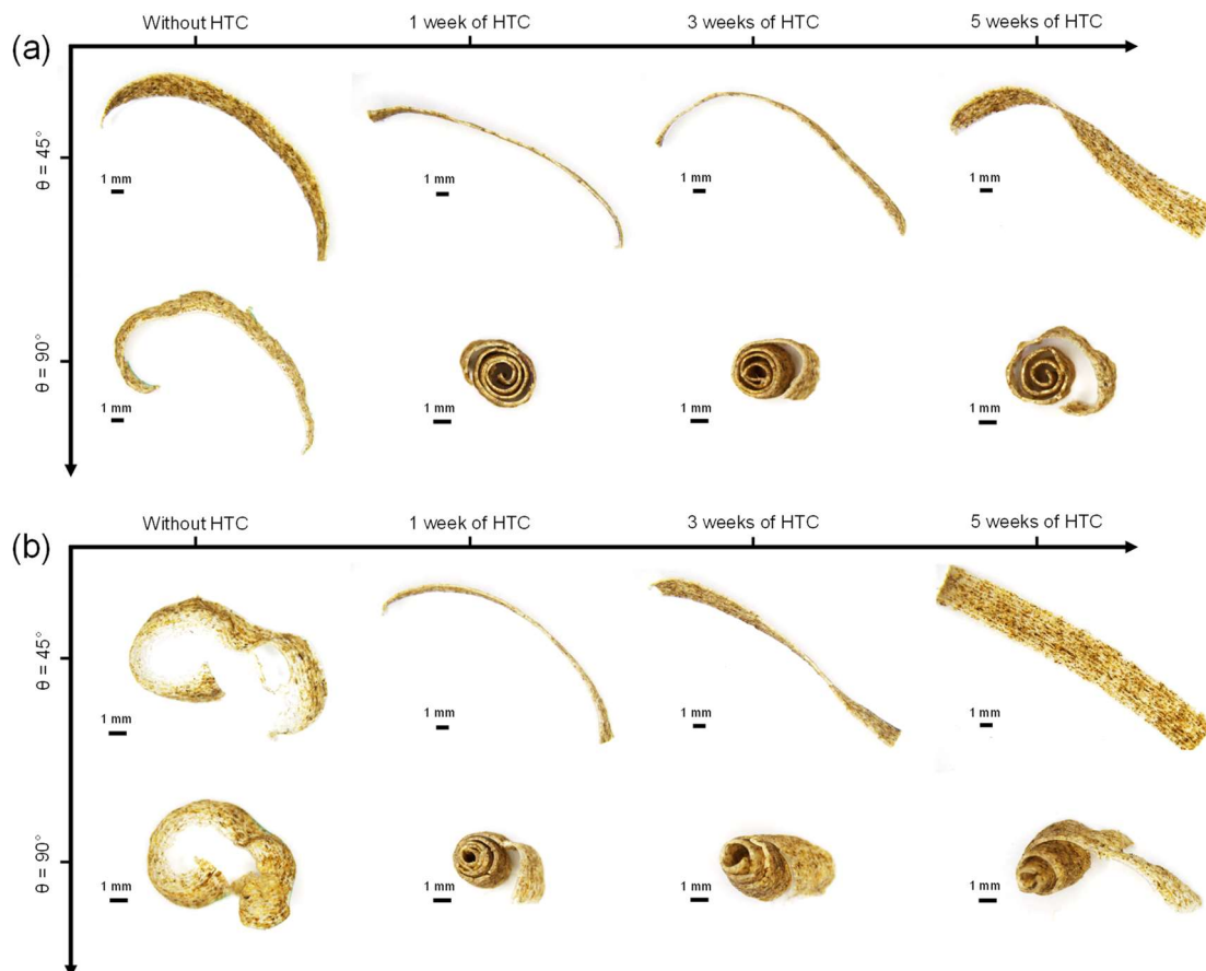
Figure 5: Shape of the formed flax/PLA chips under hygrothermal conditioning at (a) T=30^\circ\text{C} and (b) T=60^\circ\text{C}
