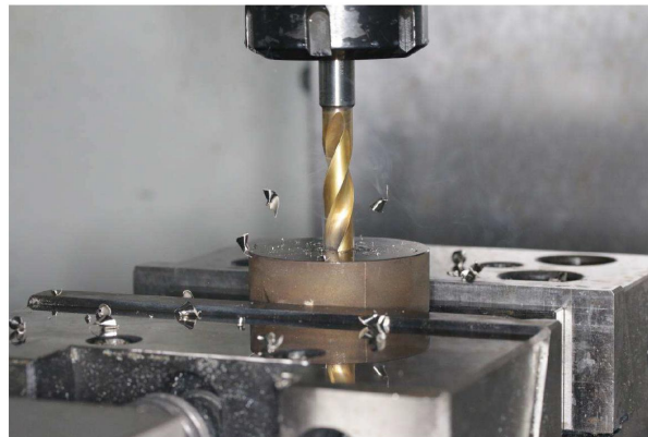
Figure 3. Experimental setup during the dry drilling tests.
