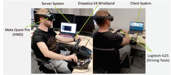
Fig. 3. Experimental setup for the study with Meta Quest Pro head-mounted display (HMD) and Empatica E4 wristband attached to a participant.
