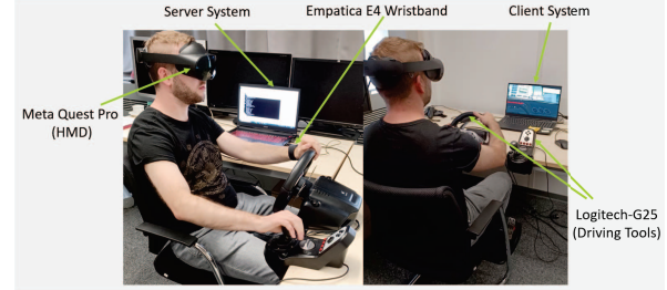
Fig. 3. Experimental setup for the study with Meta Quest Pro head-mounted display (HMD) and Empatica E4 wristband attached to a participant.
