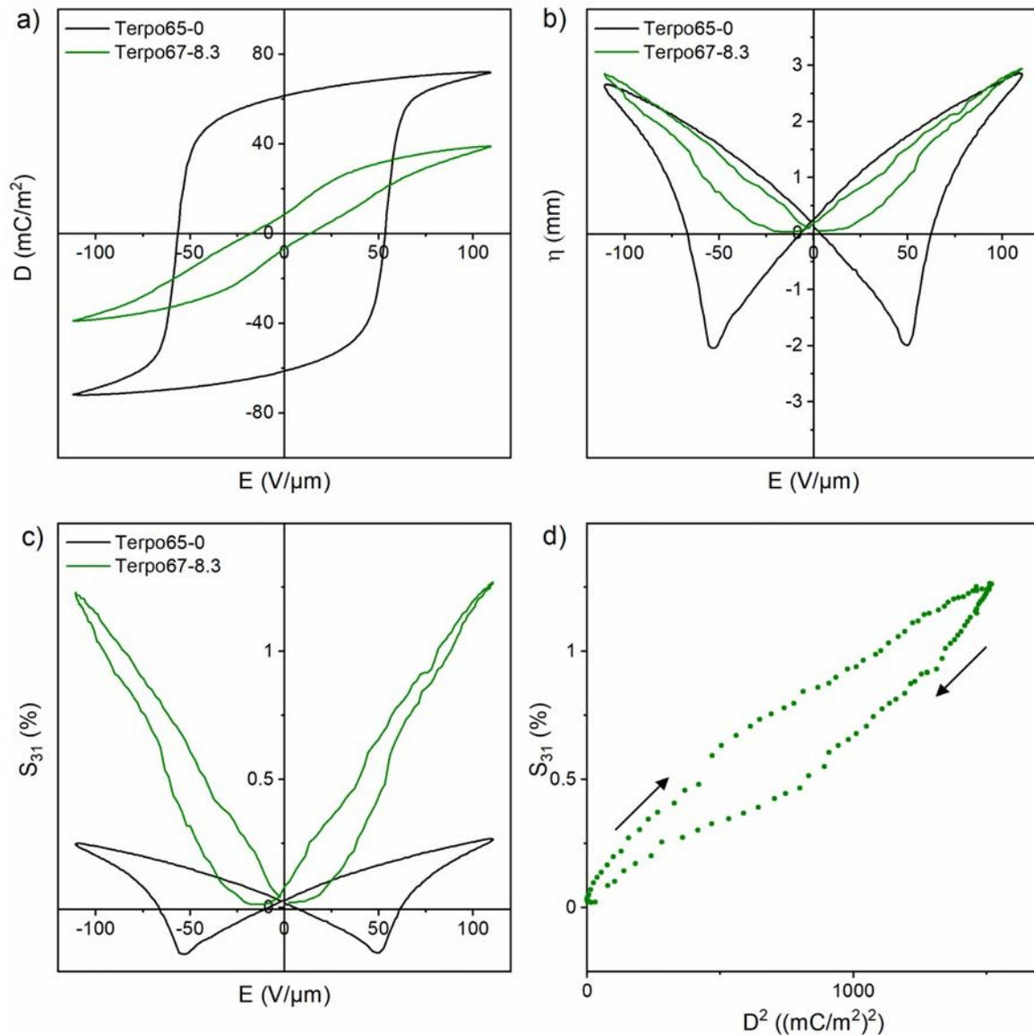
**Figure 2:** a) Electric displacement-electric field ( $D$ - $E$ ) loops, b) deflection-electric field ( $\eta$ - $E$ ) loops, and c) cross deformation-electric field ( $S_{31}$ - $E$ ) loops for Terpo65-0 and Terpo67-8.3 actuators. d) Evolution of  $S_{31}$  with respect to  $D^2$  for Terpo67-8.3.
