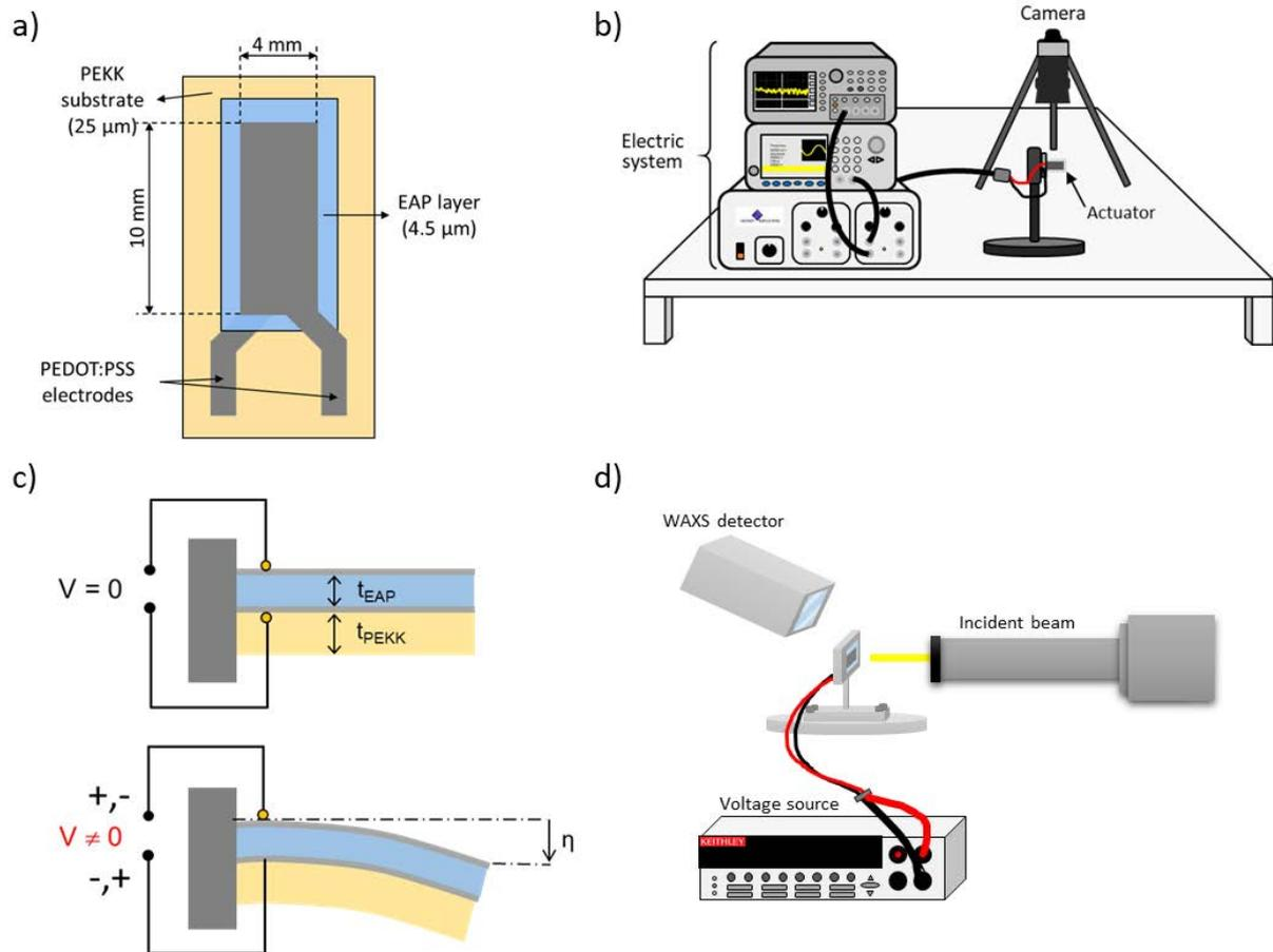
**Figure 1:** a) Scheme of the actuator with its layers (top view), b) experimental setup for the measurement of the macroscopic deflection of the actuator, c) scheme of the cross-section of the actuator before and during the application of an external electric field, and d) experimental setup for the in-situ WAXS analyses at Soleil synchrotron.
