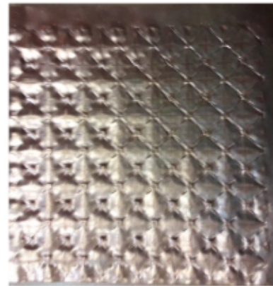
Fig. 5. Workpiece after two passes of the RCS.
