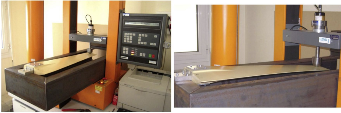
Fig. 4 Bending test on the blades
