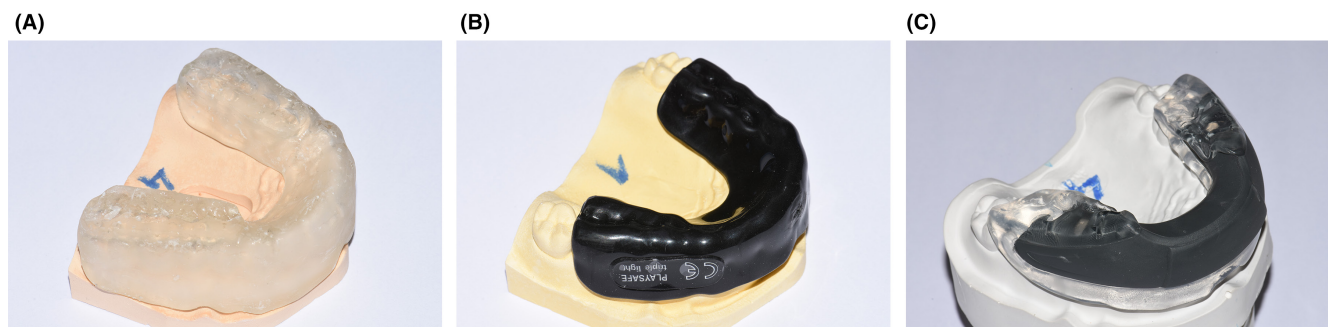
FIGURE 1 Views of tested mouthguards: (A) custom-made 3D-printed mouthguard (3DMG), (B) custom-made thermoformed mouthguard (TMG), and (C) industrial mouthguard (IMG).
