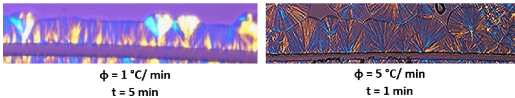
FIGURE 8 The different morphologies observed at the fiber/matrix interface as a function of the cooling rate.
