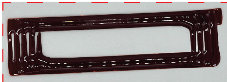
Figure S7: Photographs of as-printed PF resin with pTSA with respective wait time to show the surface finish of the final product.
