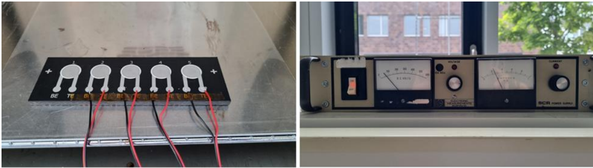
Figure 2: Polarization of PZT sensors on CFRP test samples
